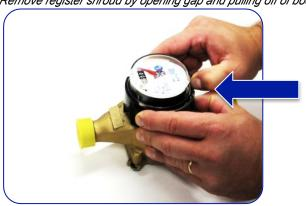
**Step 6:** *Meter with register and housing removed*
