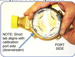
**Step 2:**Twist clockwise until mechanical stop.
