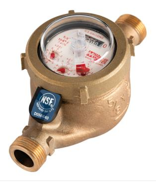
Velocity-type meter meeting or exceeding the performance requirements of AWWA Standard C-708. Water, evenly distributed through multiple inlet ports, flows past an impeller in the measuring chamber, creating an impeller velocity directly proportional to water flow rate.
