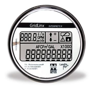
This GridLinx<sup>™</sup> AMI universal endpoint replaces an existing meter's register to take advantage of the life left in your utility's existing water meters while providing robust communication and seamless integration of Master Meter and other water meters into the Landis+Gyr Gridstream network.
