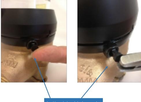
Locking pin is pointed upward
