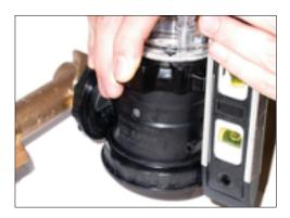
Turn locking nut clockwise to loosen.
