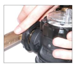
3. Position FAM Measuring Unit to Flow Tube; be sure the Measuring Unit is seated properly when mated with Flow Tube and that it is vertically level.
