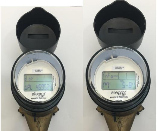
After approx. 10 gallons of water has run through the meter, the display will show the current reading.
