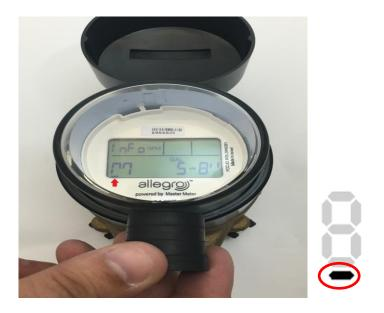
Once unit has been activated with magnet, the display screen will scroll through the following images.
