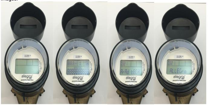
After the register has been activated and has scrolled through the four screens above, the register will toggle between the UPLINK frequency and the size the register is programmed for.
