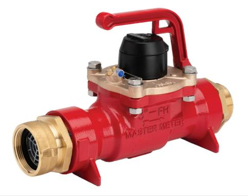
A lightweight aluminum case, replaceable and lockable handle, stainless steel internal inlet strainer, and unitized measuring chamber simplify handling and maintenance for the Master Meter Fire Hydrant Meter. The 3" FHM boasts high accuracy over broad flow ranges to maximize revenue from construction site or other temporary water use.
