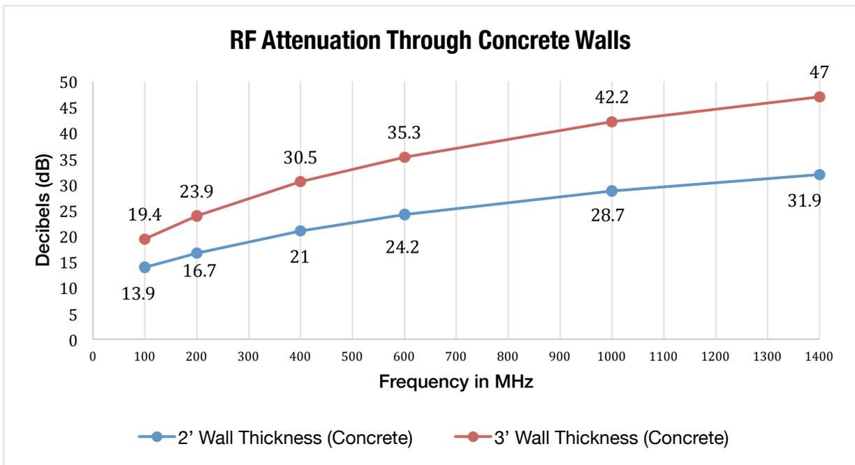
**Figure 1:** RF attenuation through concrete walls (adapted from Phillips Laboratories "Measurement of RF Propagation into Concrete Structures over the Frequency Range 100 MHz to 3 GHz")
