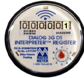
Figure 2: Interpreter Register reading in 10 USG
