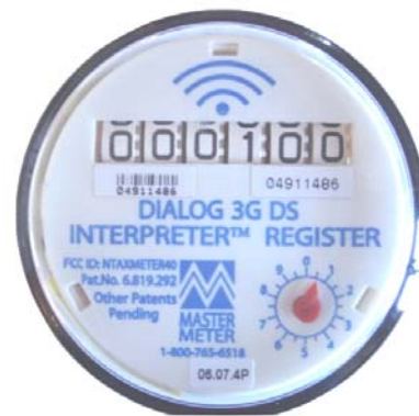
Figure 6: Interpreter Register reading 10 USG with Test Mode division at 100.
